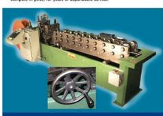
The E-Stud Line was developed by Custom Rollform Products as an Economical System to manufacture Stud and Track on a just-in-time basis. It offers the latest concepts in quick-change set-ups that allow you to convert from Stud to Track in less than a minute. This allows manufacturers of Pre-fabricated Housings and Major Contractors to produce cut-to-length sections On-time and as needed without hours of Set-ups, Coil Changes and Excessive Scrap Loss.
