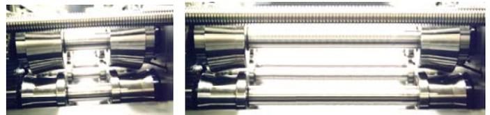
Our Variable Width Rollform design positions the roll tooling with a simple leadscrew handwheel. The variable tooling design allows the operator to make width changeovers in less than one (1) minute.
