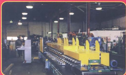
Coil Strip Feed, Gasket Feed, Punch/Notch, Rollform, Toggle-Lock & Cut-To-Length System
