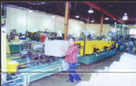
Completed 3-sided wrapper laterally ejected out of Tangent Former.
